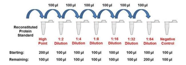
For samples of unknown protein concentrations, serial dilute the experimental sample using Standard & Sample Diluent to determine range
